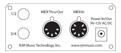
1/2 and 3/4 – These jacks connect to the footswitch or external switching jacks of your amplifier or other device. The tip conductor of the 1/2 jack is controlled by the 1 button on the front panel, and the ring conductor is controlled by the 2 button. Likewise, the tip of the 3/4 jack is controlled by the 3 button and the ring is controlled by the 4 button.
